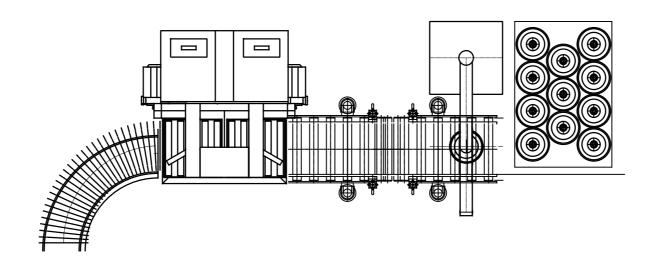
Semi Auto 2 head with in-feed roller and out-feed straight roller with vacuum lifter
